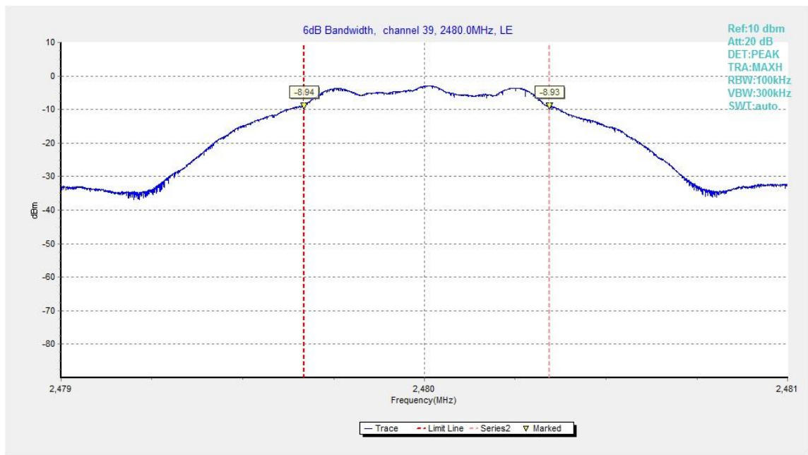
Fig.22. 6dB Bandwidth: GFSK, 2480 MHz
