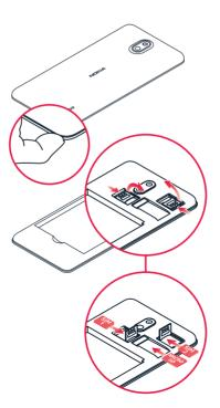
**Note:** Switch the device off and disconnect the charger and any other device before removing any covers. Avoid touching electronic components while changing any covers. Always store and use the device with any covers attached.
