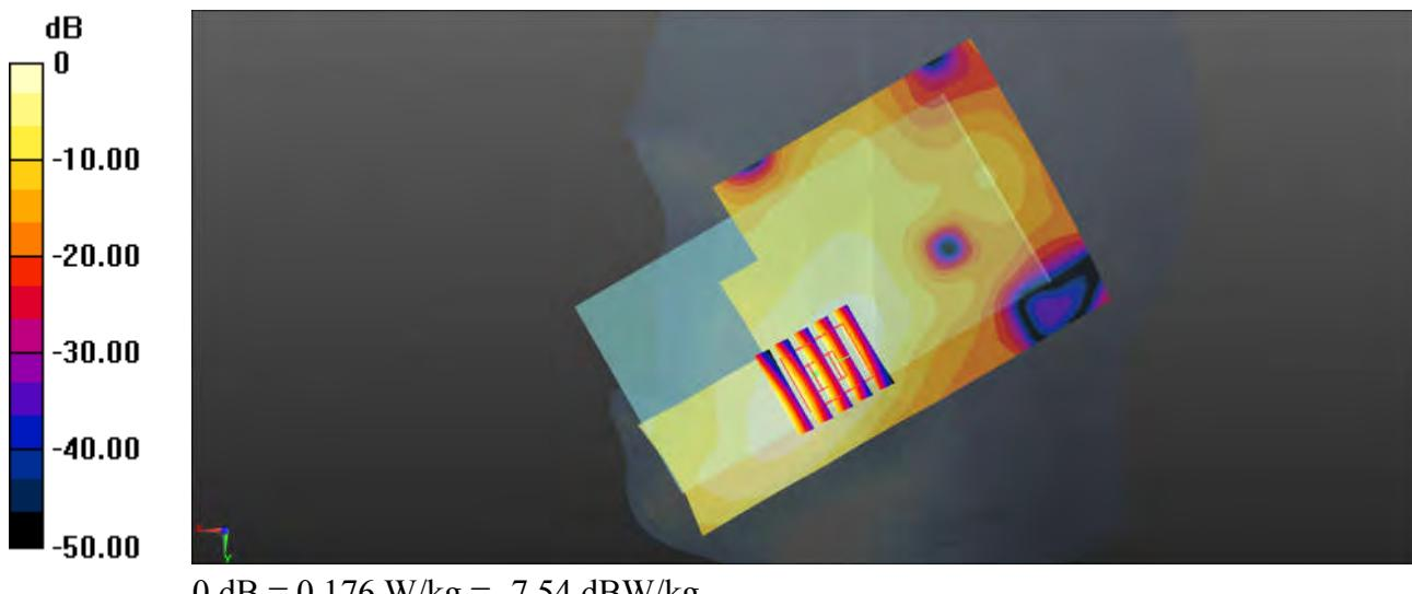
**07\_LTE Band 5\_10M\_QPSK\_1RB\_25Offset\_Right Cheek\_0mm\_Ch20525**
