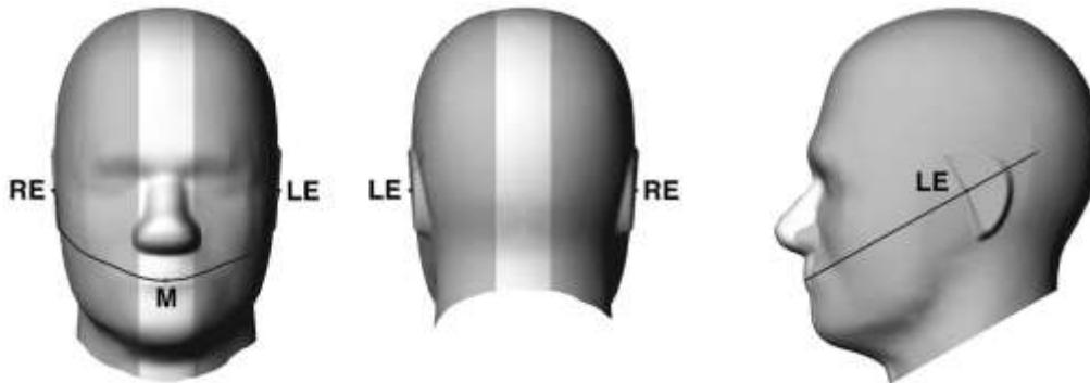
Fig 11.1.1 Front, back, and side views of SAM twin phantom
