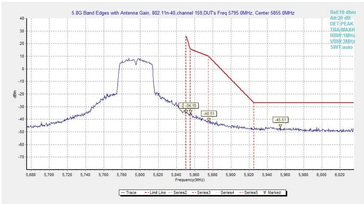
Fig. 46 Band Edges (802.11n-HT40, 5795MHz)
