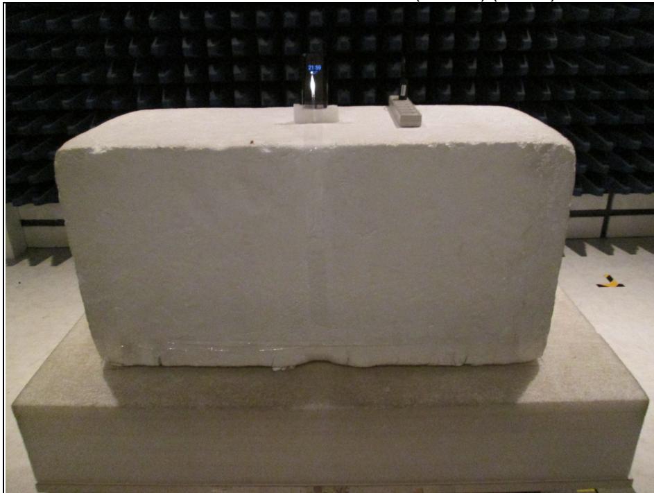
Radiated Emission Test above 1GHz (WWAN) (Z-Axis)
