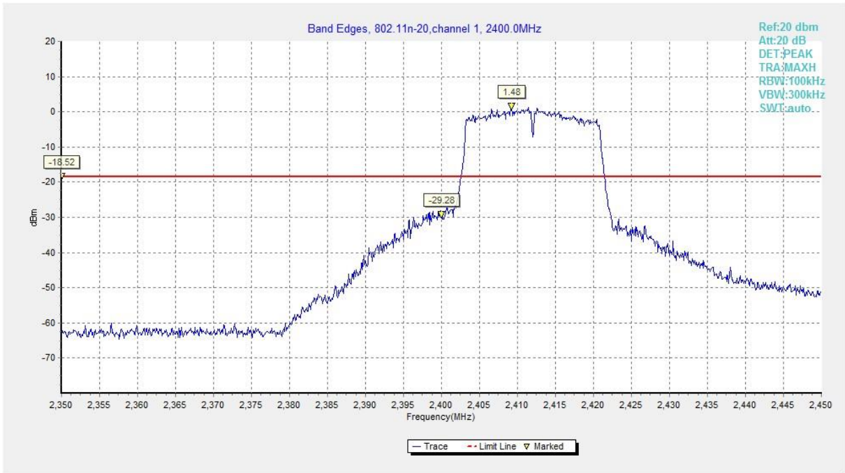
Fig.A.5.5 Band Edges (802.11n-HT20, Ch 1)
