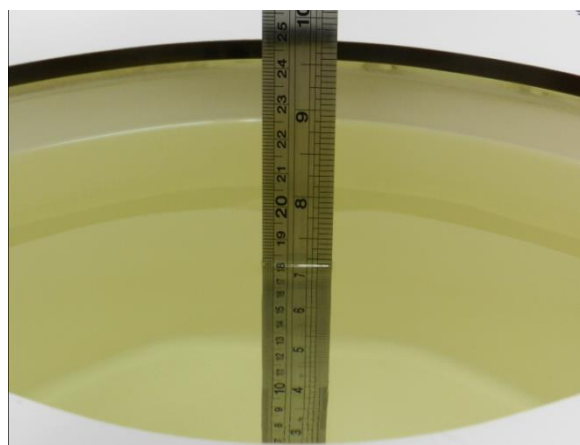
Fig 10.2 Photo of Liquid Height for Body SAR
