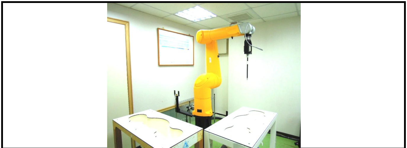
Fig-3.3 DASY5 Measurement System
