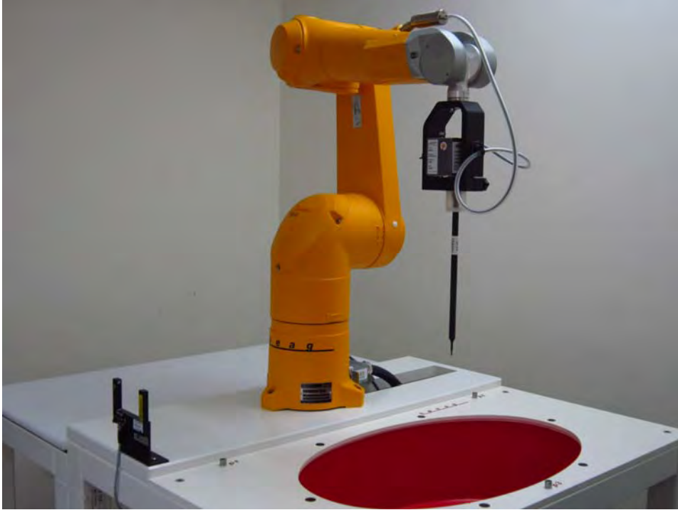
Fig.1 Photograph of the SAR measurement system
