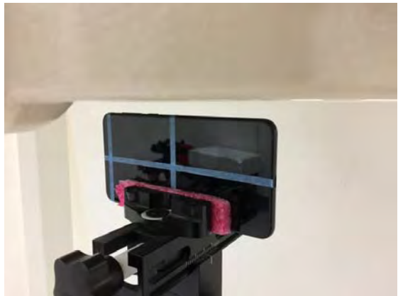
Fig.13 EUT Right side to flat phantom
