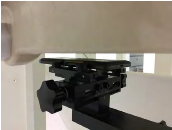
Fig.10 EUT Back side to flat phantom
