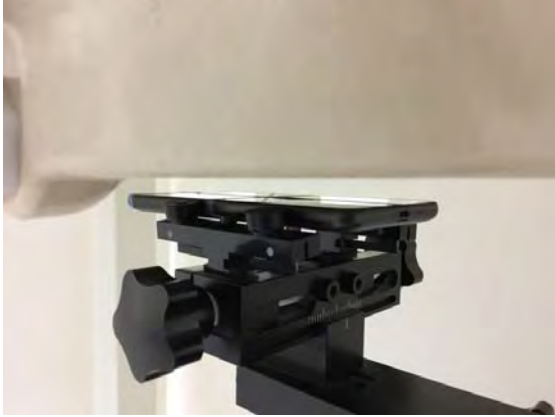
Fig.9 EUT Front side to flat phantom
