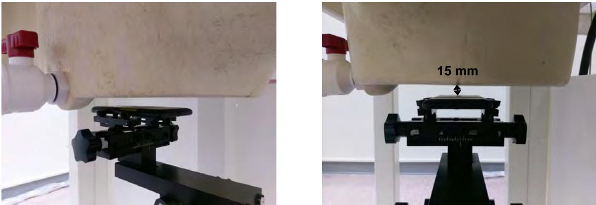
Fig.8 EUT Back side to flat phantom
