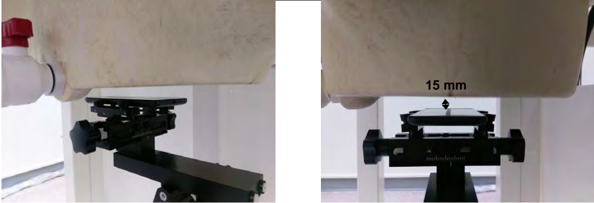
Fig.7 EUT Front side to flat phantom
