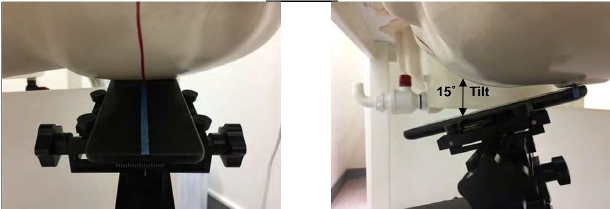
Fig.6 Left Head Section / Ear-Tilt Position(15°)
