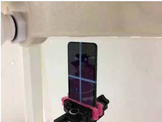
Fig.11 EUT Bottom side to flat phantom
