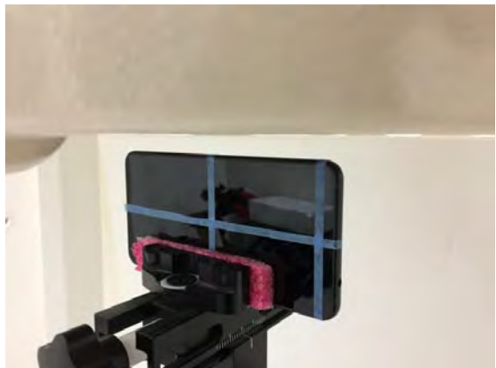
Fig.14 EUT Left side to flat phantom
