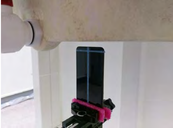
Fig.12 EUT Top side to flat phantom
