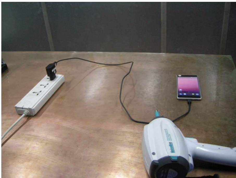
Pic.4 Immunity to electrostatic discharge
