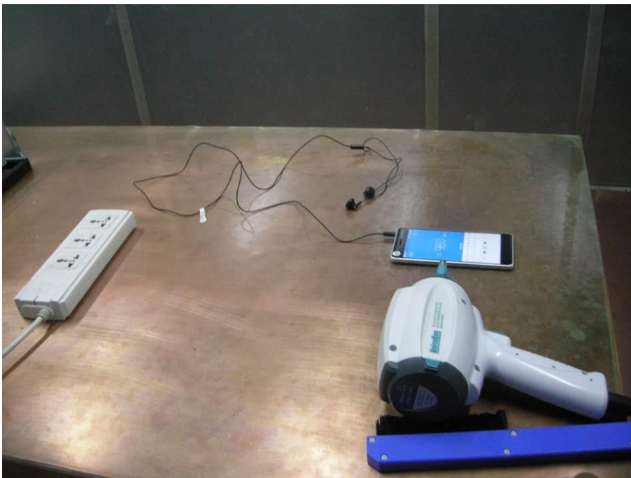
Pic.10 Immunity to electrostatic discharge (FM)
