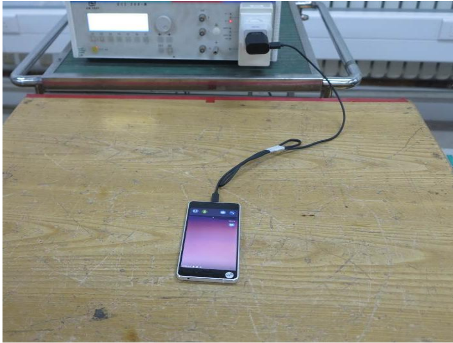
Pic.9 Immunity to voltage dips, short interruptions and variations
