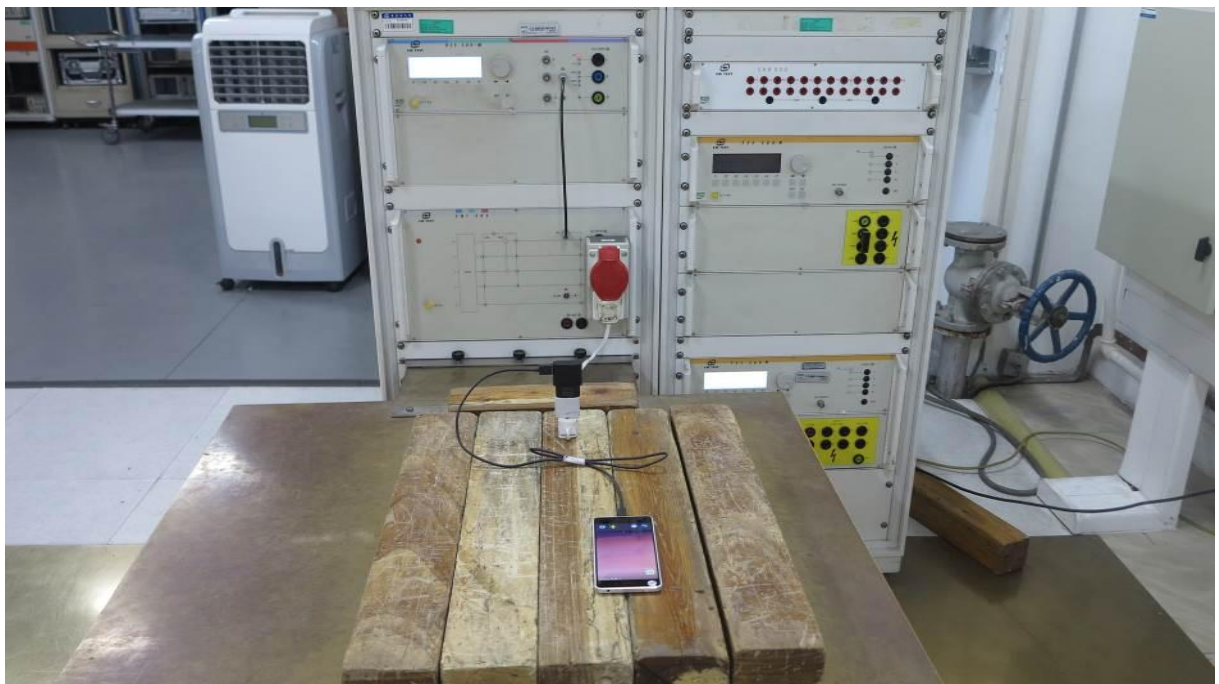
Pic.6 Immunity to electric fast transients
