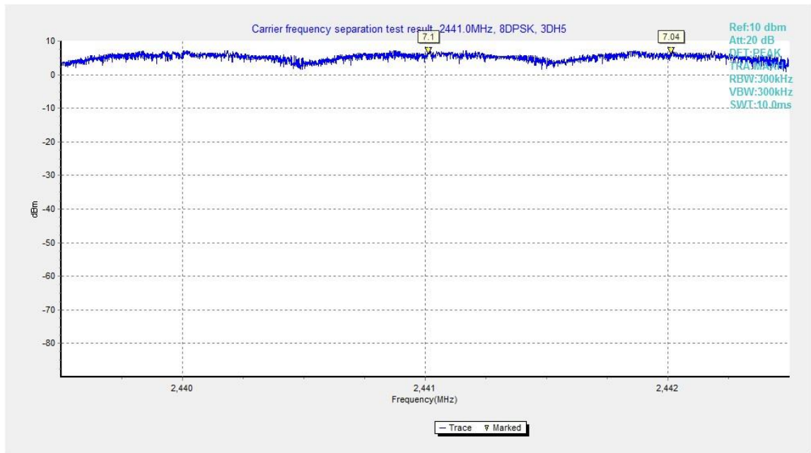
Fig.117. Carrier frequency separation measurement: 8DPSK, Channel 39
