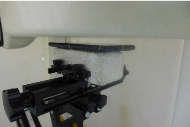
Front, Test Separation 10 mm
