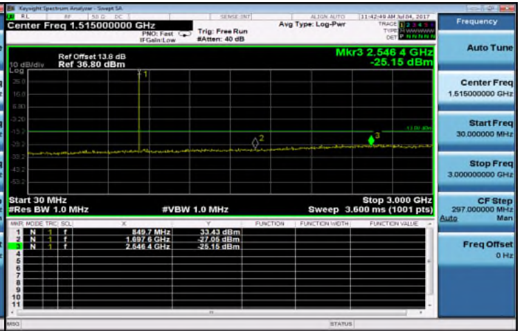
Out of Band Emission Low_GPRS_850MHz_LowCH128-824.2
