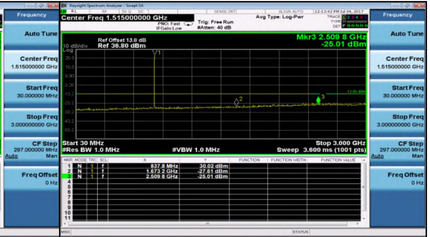
Out of Band Emission Low_EDGE_850MHz_HighCH251-848.8
