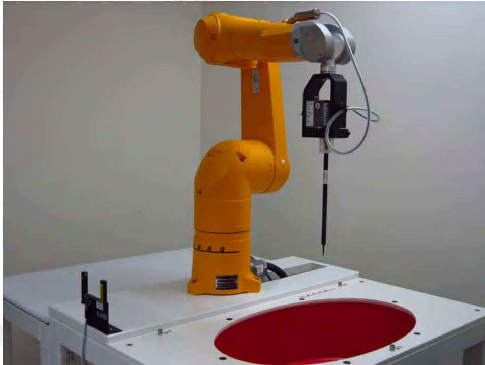
Fig.1 Photograph of the SAR measurement system
