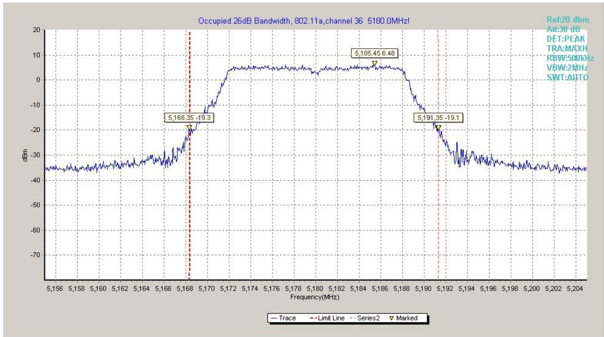
Fig. 1 Occupied 26dB Bandwidth (802.11a, 5180MHz)
