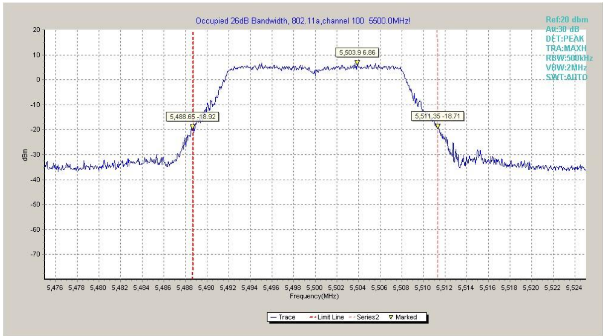
Fig. 7 Occupied 26dB Bandwidth (802.11a, 5500MHz)
