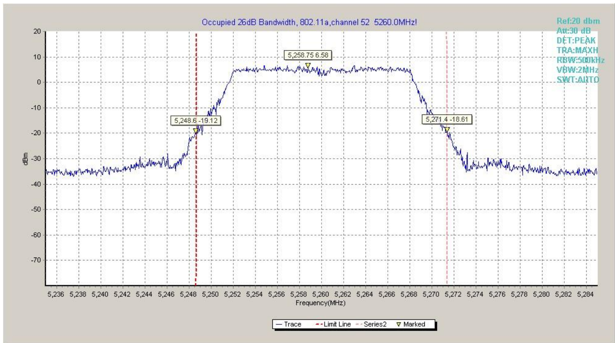
Fig. 4 Occupied 26dB Bandwidth (802.11a, 5260MHz)
