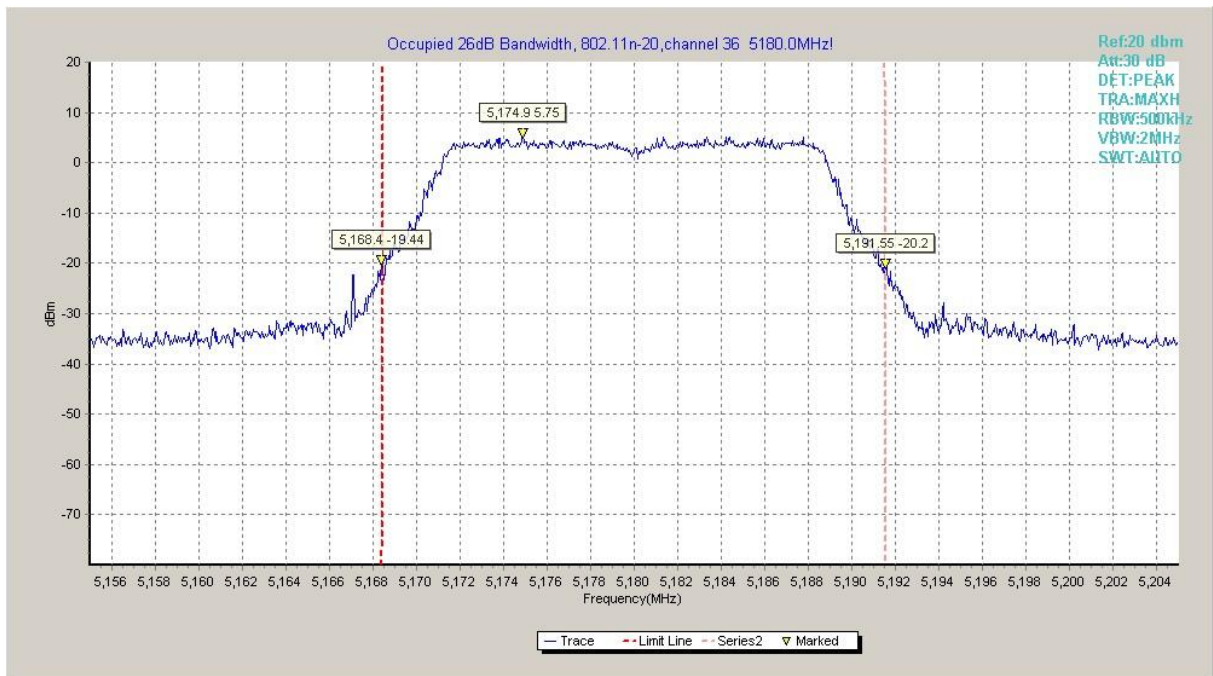
Fig. 10 Occupied 26dB Bandwidth (802.11n-HT20, 5180MHz)
