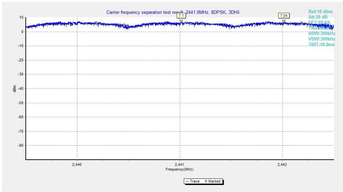
Fig.117. Carrier frequency separation measurement: 8DPSK, Channel 39
