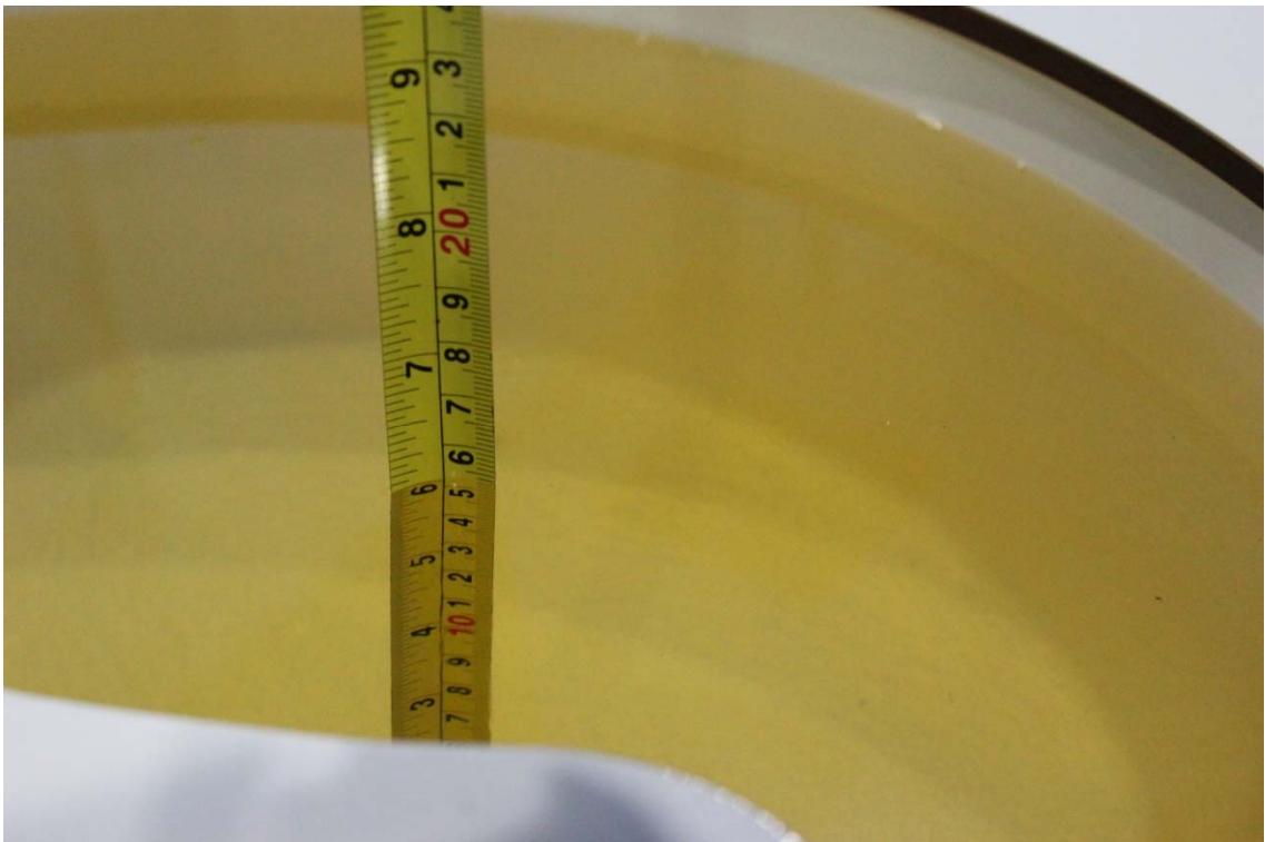
Picture 7-2 Liquid depth in the Flat Phantom (750 MHz)
