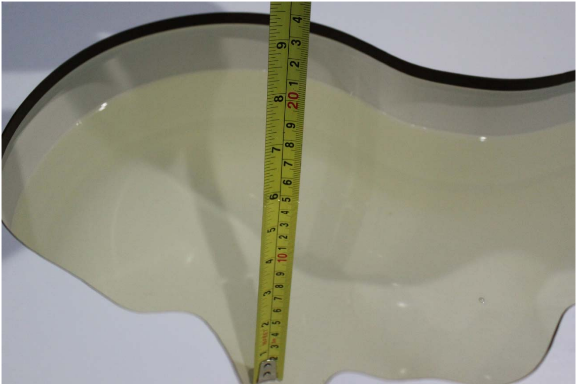
Picture 7-13 Liquid depth in the Head Phantom (5GHz)
