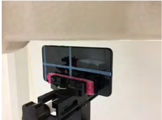
Fig.13 EUT Right side to flat phantom
