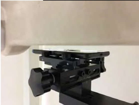
Fig.9 EUT Front side to flat phantom
