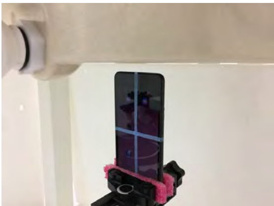
Fig.11 EUT Bottom side to flat phantom
