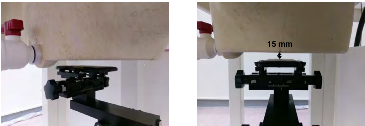
Fig.8 EUT Back side to flat phantom
