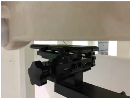
Fig.10 EUT Back side to flat phantom
