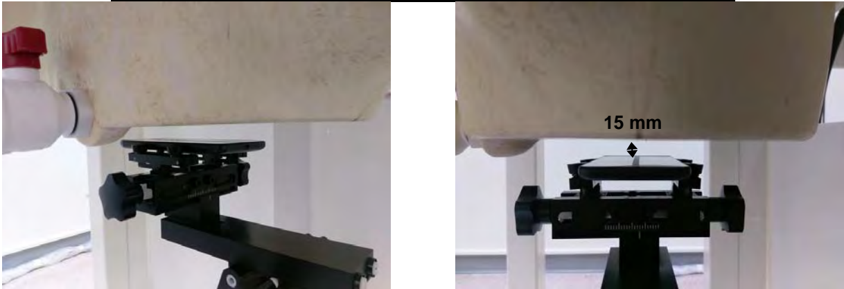
Fig.7 EUT Front side to flat phantom
