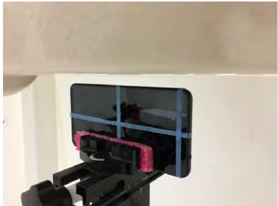
Fig.14 EUT Left side to flat phantom
