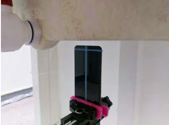
Fig.12 EUT Top side to flat phantom
