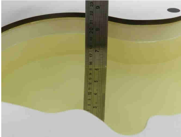
Fig 10.1 Photo of Liquid Height for Head SAR
