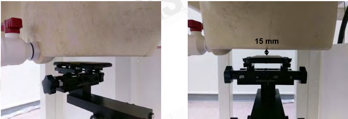
Fig.8 EUT Back side to flat phantom
