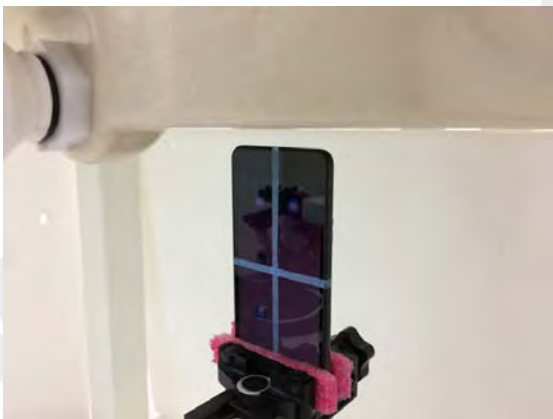
Fig.11 EUT Bottom side to flat phantom
