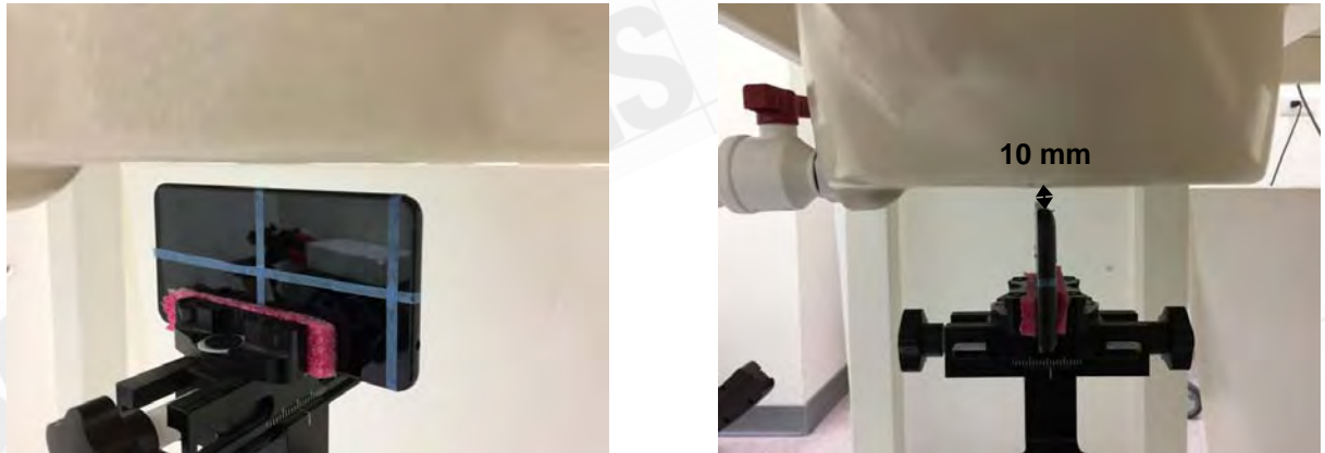
Fig.14 EUT Left side to flat phantom
