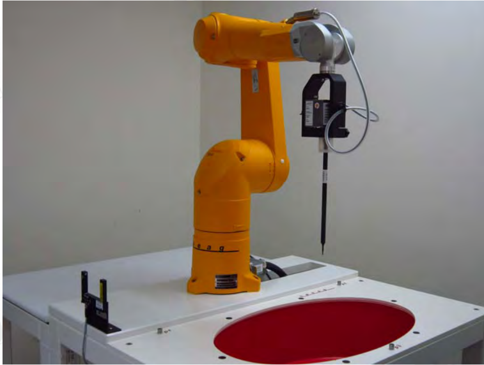
Fig.1 Photograph of the SAR measurement system
