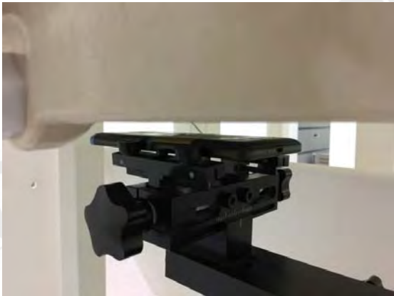
Fig.10 EUT Back side to flat phantom
