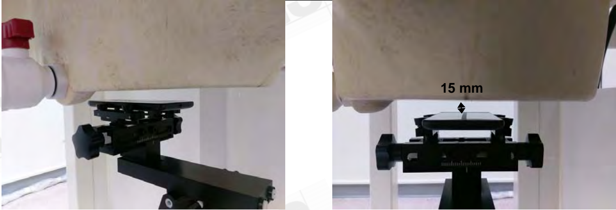
Fig.7 EUT Front side to flat phantom
