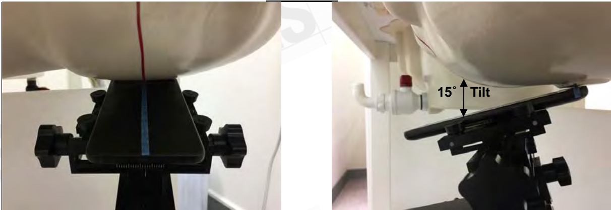
Fig.6 Left Head Section / Ear-Tilt Position(15°)
