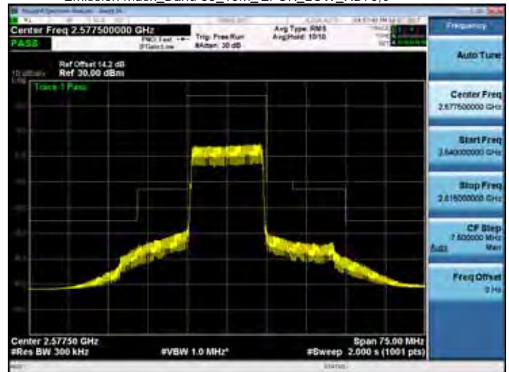
Emission Mask_Band 38_15M_QPSK_MID_RB1,0
