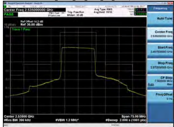
Emission Mask_Band 7_20M_QPSK_HIGH_RB1,0
