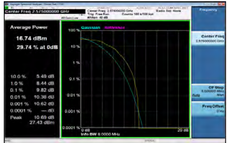
10MHz BW LTE-Band 38(16QAM Number: 50 Offset: 0) Channel Low
