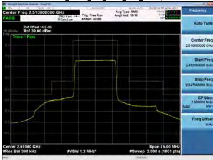
Emission Mask_Band 7_20M_QPSK_MID_RB1,0
