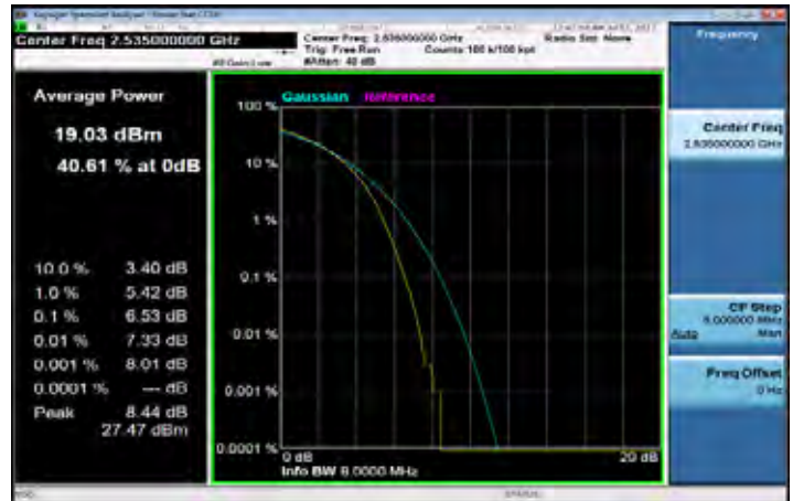
20MHz BW LTE-Band 7(16QAM Number: 100 Offset: 0) Channel Mid
