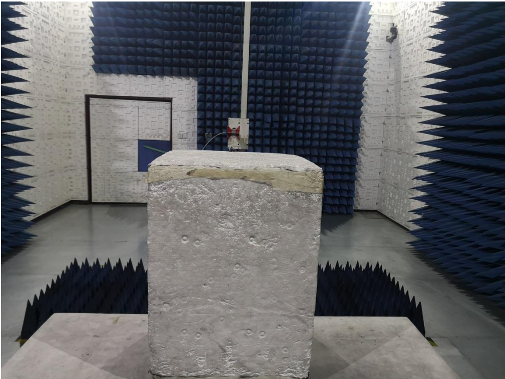
RADIATED EMISSION TEST SETUP ABOVE 1GHz
