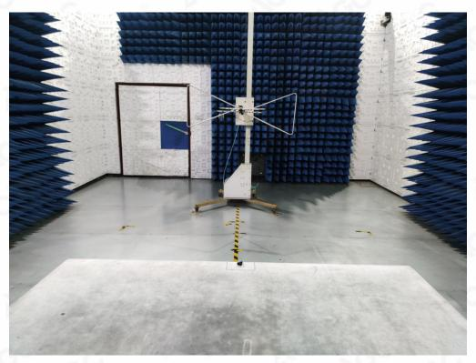
RADIATED EMISSION TEST SETUP ABOVE 1GHz
