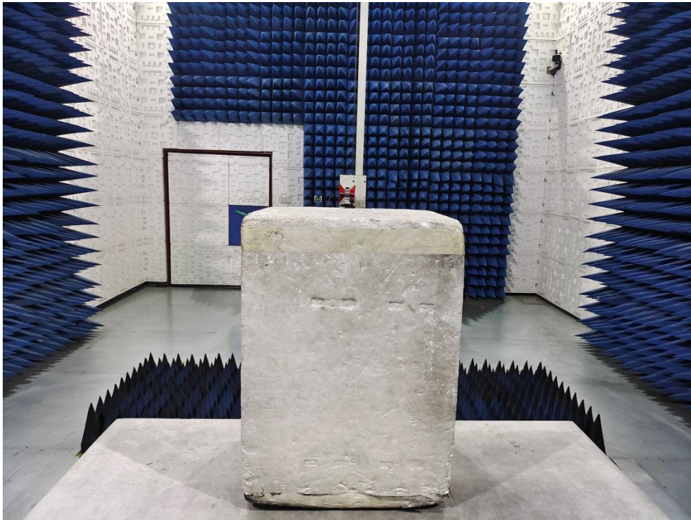
RADIATED EMISSION TEST SETUP ABOVE 1GHz
