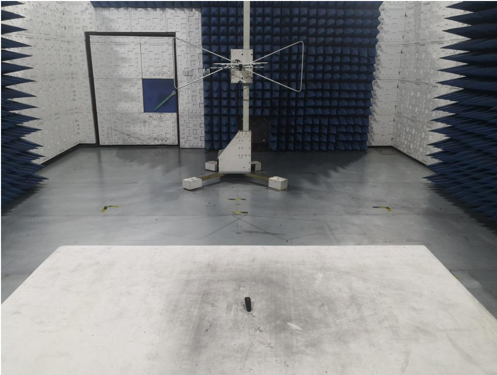
RADIATED EMISSION TEST SETUP ABOVE 1GHz
