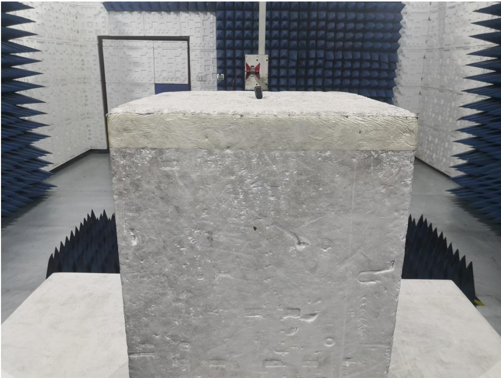
RADIATED EMISSION TEST SETUP ABOVE 1GHz
