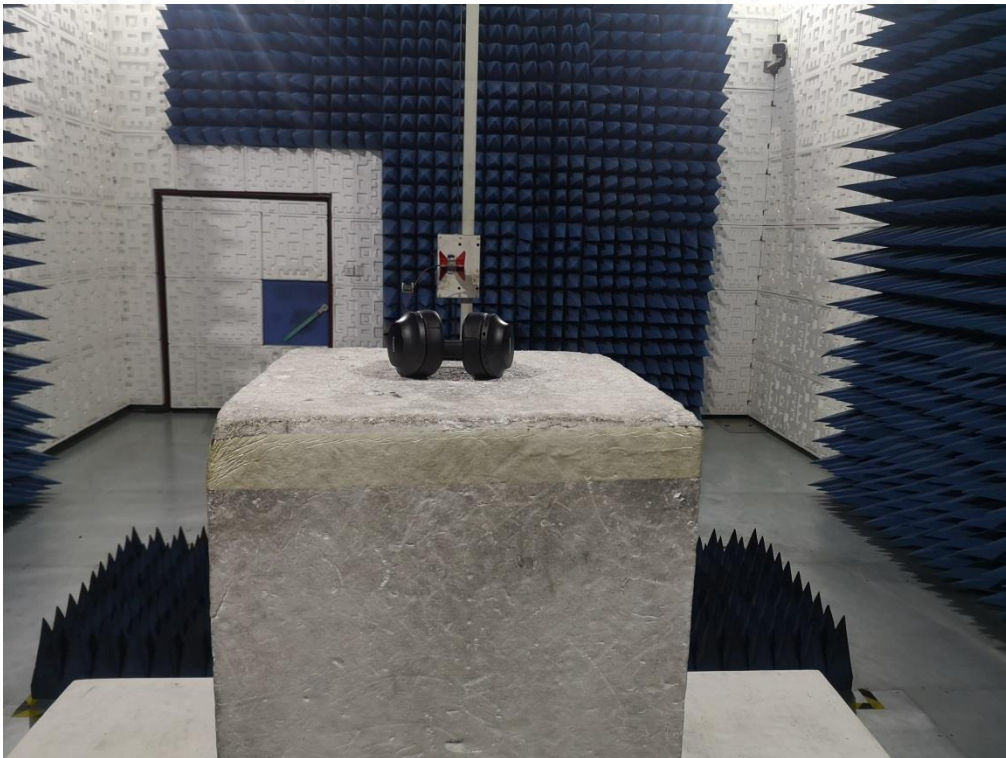
RADIATED EMISSION TEST SETUP ABOVE 1GHZ
