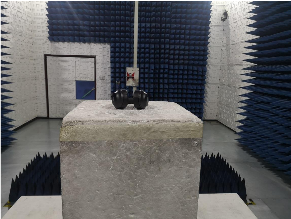
RADIATED EMISSION TEST SETUP ABOVE 1GHz
