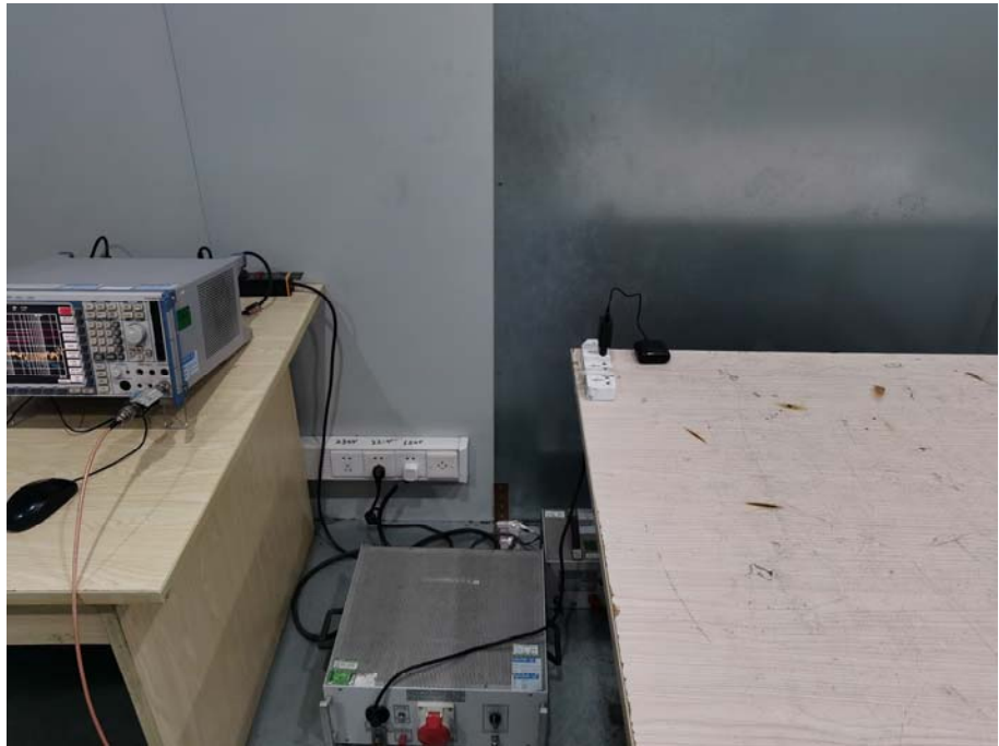
Conducted Emission Test Setup
