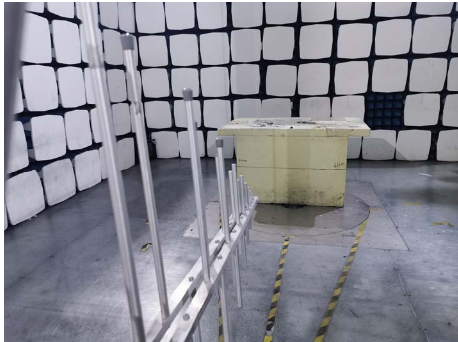
Radiation Emission Test Setup (30MHz to 1GHz)
