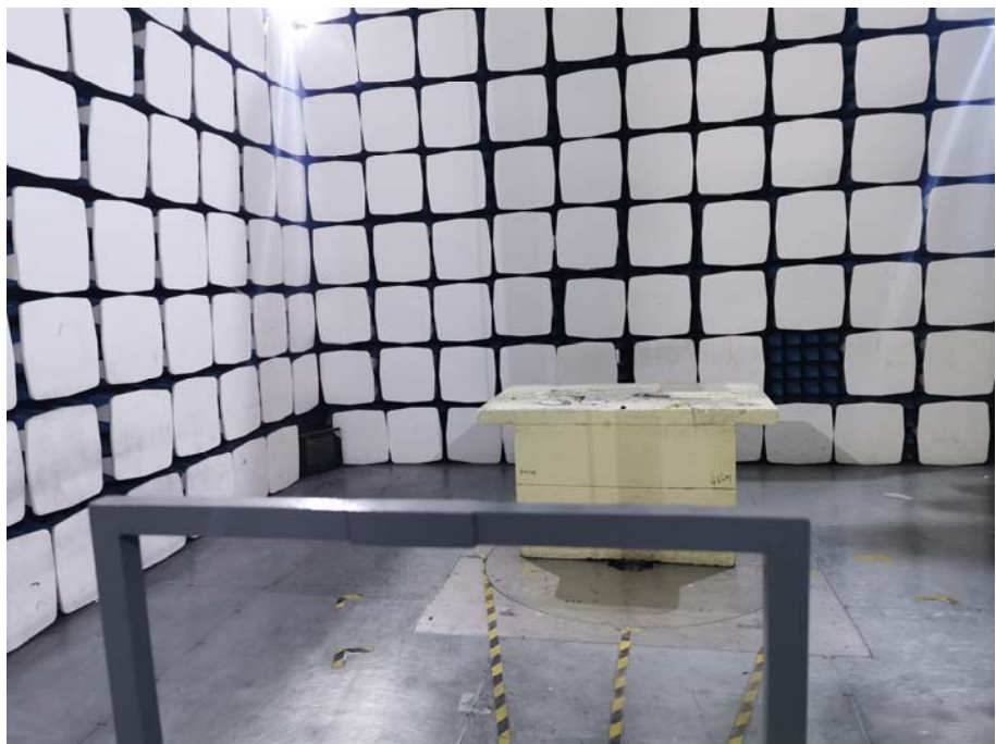
Radiation Emission Test Setup (Below 30MHz)
