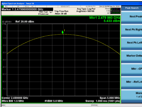
Peak output Power plot on channel 78 (3Mbps)
