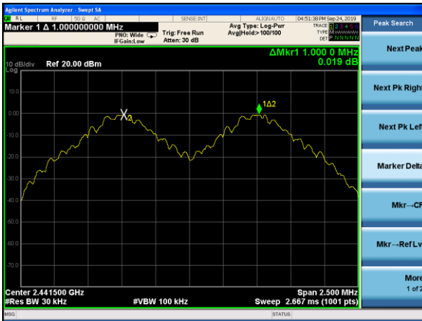
(1Mbps) Channel Separation plot on channel 77-78
