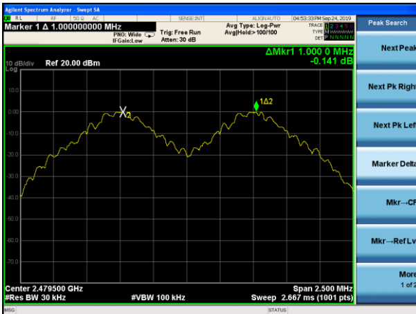
(1Mbps) Channel Separation plot on channel 77-78
