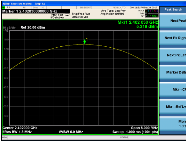
Peak output Power plot on channel 39 (3Mbps)
