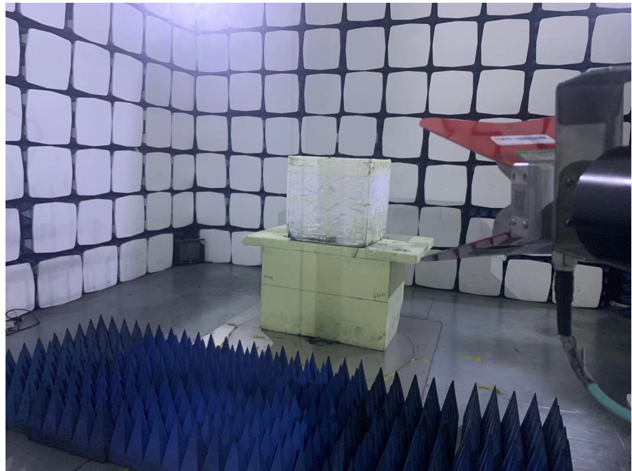
Radiation Emission Test Setup (1GHz to 18GHz)
