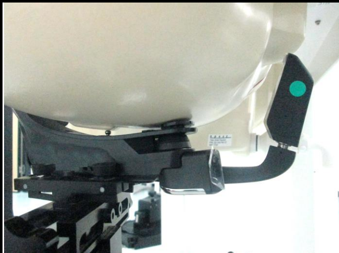
Test Position 7: Right Head (5G WLAN)
