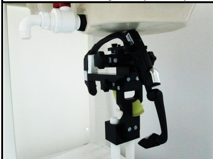
Test Position 13: Bottom Side (5G WLAN)
