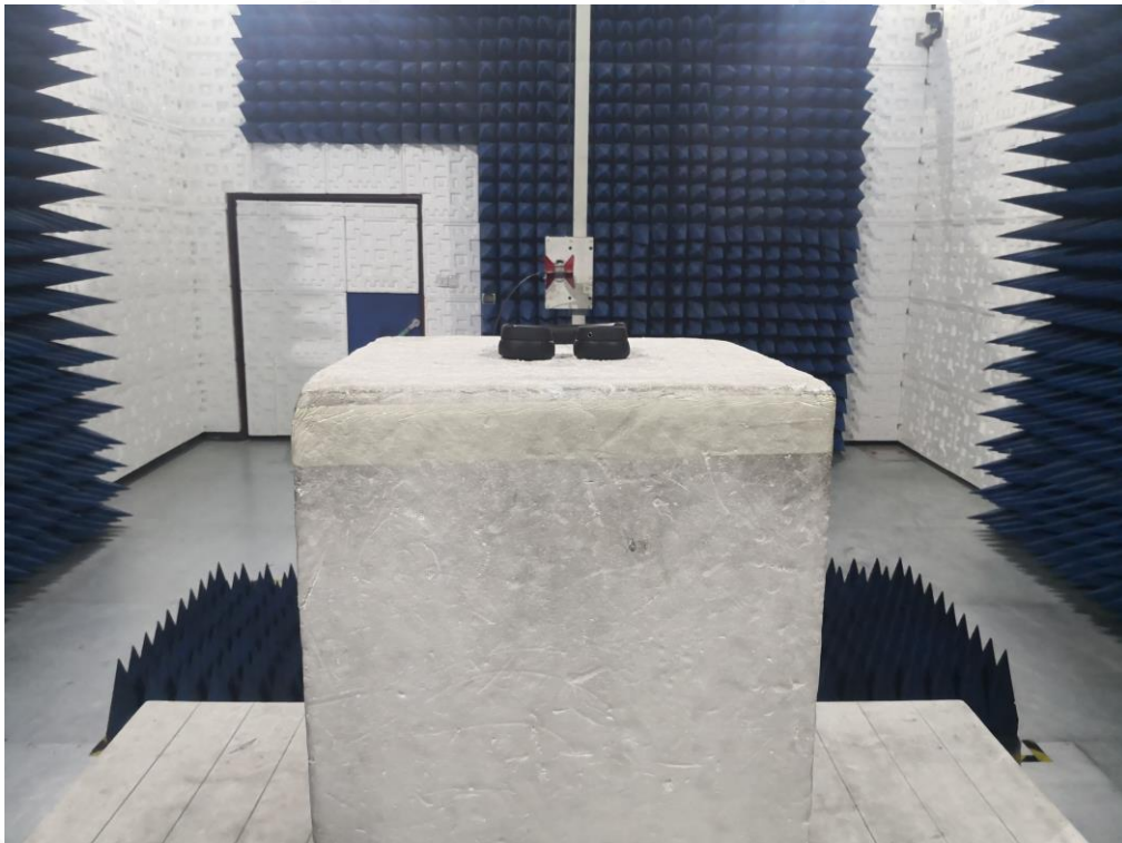
RADIATED EMISSION TEST SETUP ABOVE 1GHZ
