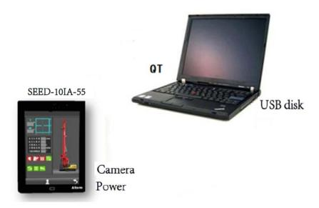
The configuration development software QT is installed on the PC. The power supply and camera are connected to the display screen, and the platform is built.
