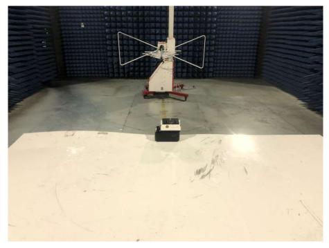
Transmitter Radiation Measurement above 1GHz
