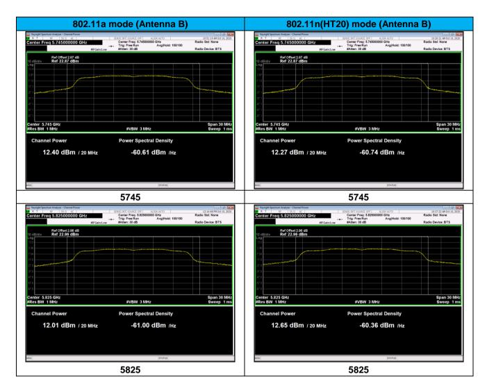
Note: We tested 802.11a/n mode the all data rate and recorded the worst case data for this channel to be 6Mbps for 802.11a mode and MCS0 for 802.11n mode.
