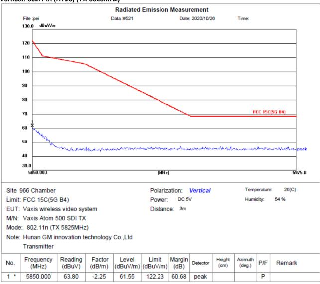
Note: We tested 802.11a/n mode the all data rate and recorded the worst case data for this channel to be 6Mbps for 802.11a mode and MCS0 for 802.11n mode.
