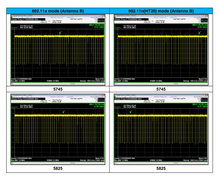
Note: We tested 802.11a/n mode the all data rate and recorded the worst case data for this channel to be 6Mbps for 802.11a mode and MCS0 for 802.11n mode.
