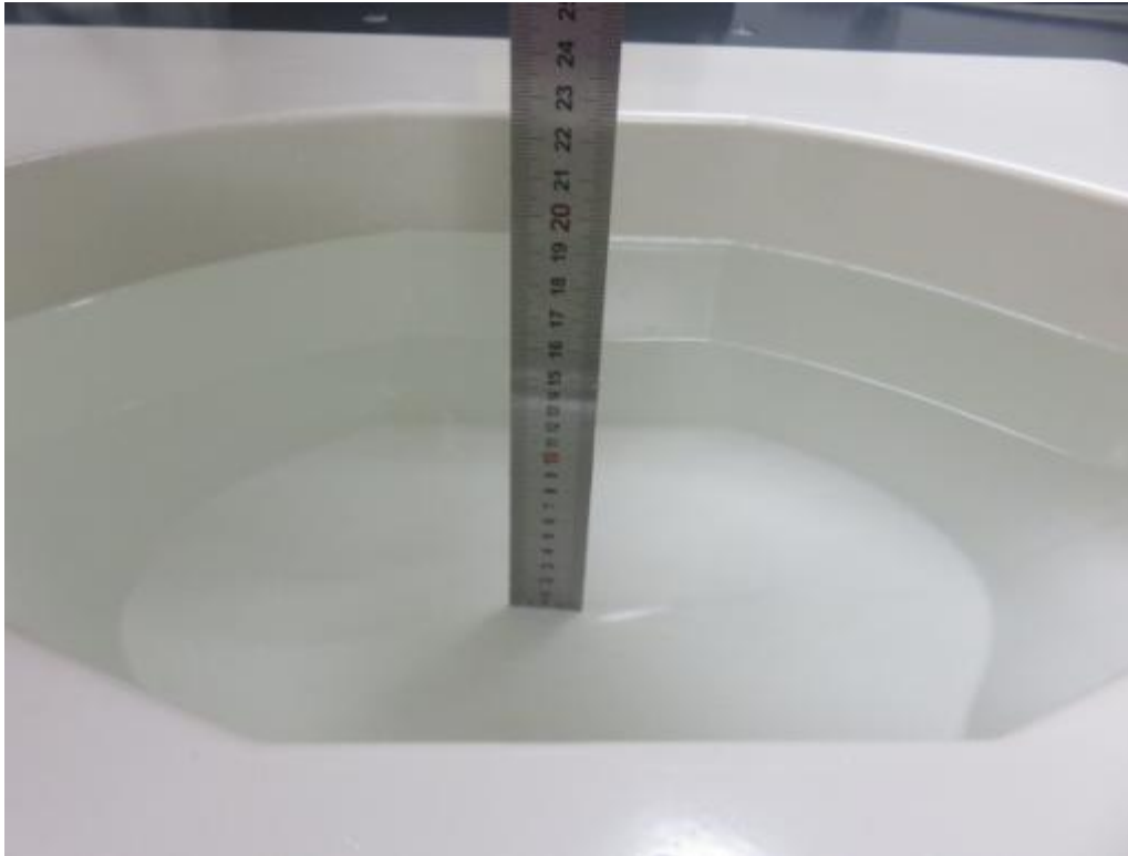
Photograph of the depth in the Body Phantom (1900MHz, 15.4 cm depth)
