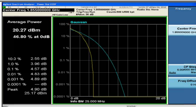
Channel Bandwidth: 10 MHz_LCH_QPSK_1RB#49
