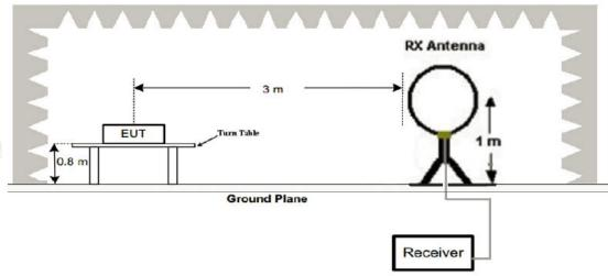
2. Radiated Emission Test-Up Frequency 30MHz~1GHz
