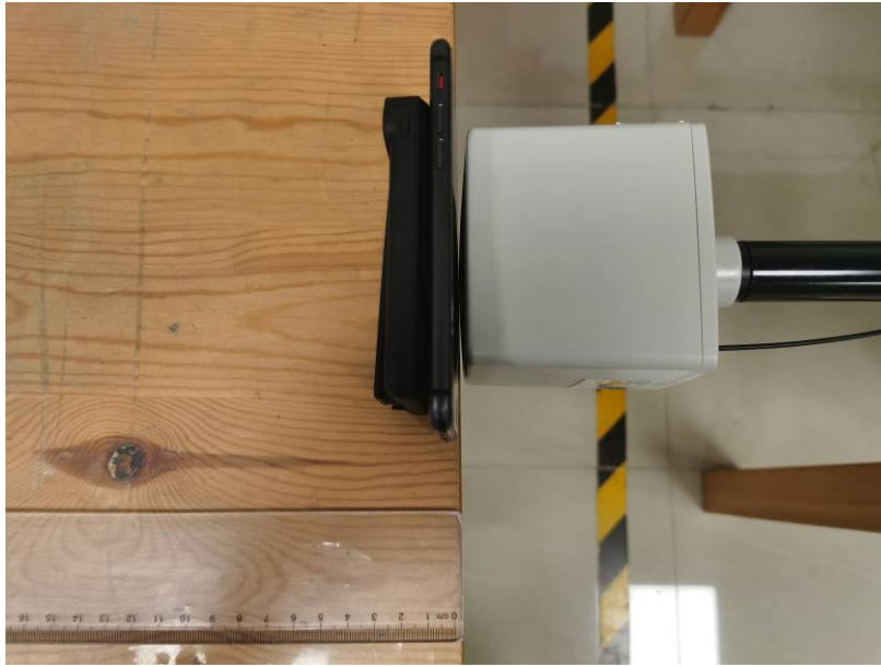
Test Position E-0cm from the edge of EUT to the geometric center of the probe
