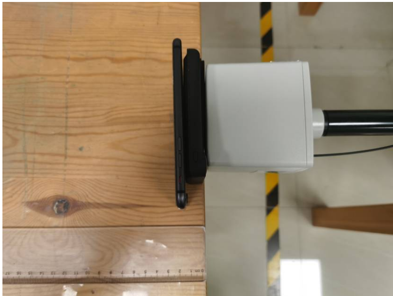
Test Position F-0cm from the edge of EUT to the geometric center of the probe
