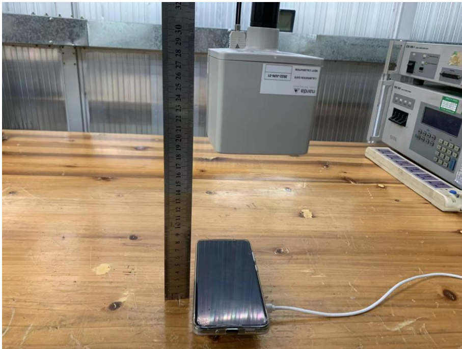
Test Position E-20cm from the edge of EUT to the geometric center of the probe
