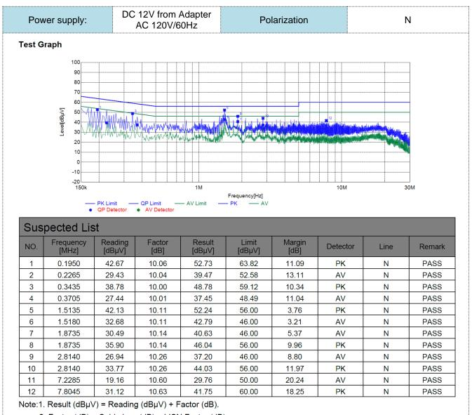
2. Factor (dB) = Cable loss (dB) + LISN Factor (dB).
