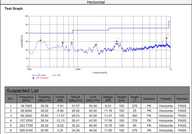
Note:1. Result  $(dB\mu V/m)$  = Reading $(dB\mu V/m)$  + Factor (dB).
