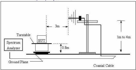
(C) Radiated Emission Test-Up Frequency Above 1GHz
