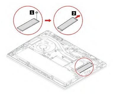
Type 2 Remove the screw and remove the M.2 solid-state drive bracket, and then remove the M.2 solid-state drive.
