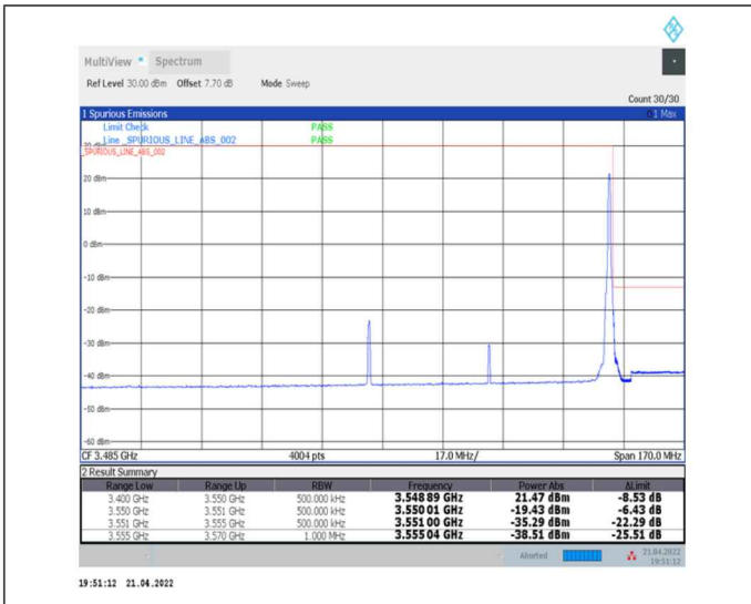
1-N78-3450-3550-30-70-H-2-DFT-PI2BPSK-Edge_1RB_Right-1@188-Ant0-PASS-see graph
