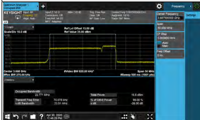
99% Occupied Bandwidth Spectrum Plot of Worst Value 20MHz+5MHz / QPSK
