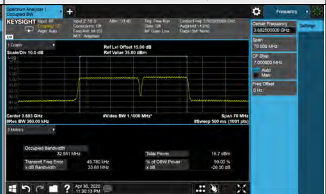
26dB Bandwidth Spectrum Plot of Worst Value 20MHz+15MHz / QPSK
