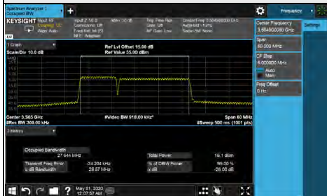
99% Occupied Bandwidth Spectrum Plot of Worst Value 10MHz+20MHz / 16QAM
