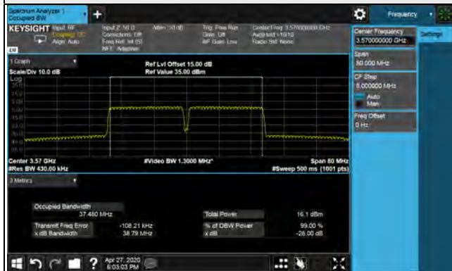
99% Occupied Bandwidth Spectrum Plot of Worst Value 20MHz+20MHz / 16QAM
