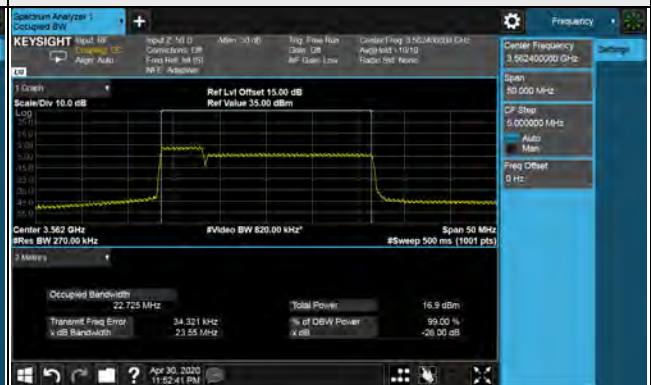
26dB Bandwidth Spectrum Plot of Worst Value 5MHz+20MHz / QPSK
