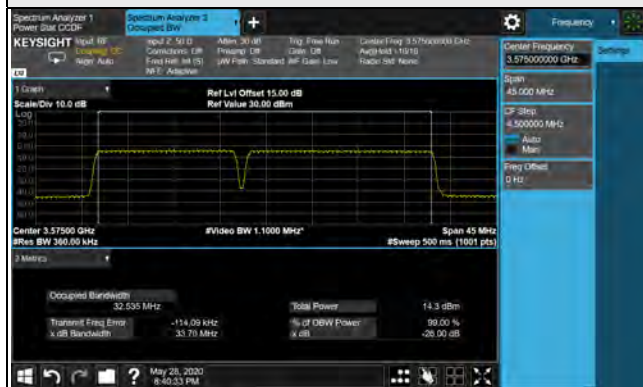
99% Occupied Bandwidth Spectrum Plot of Worst Value 15MHz+20MHz / 64QAM
